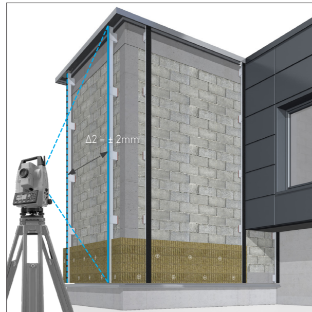
The measurement procedure checking the distances between vertical supports and determining the difference between planned and actual distances.
